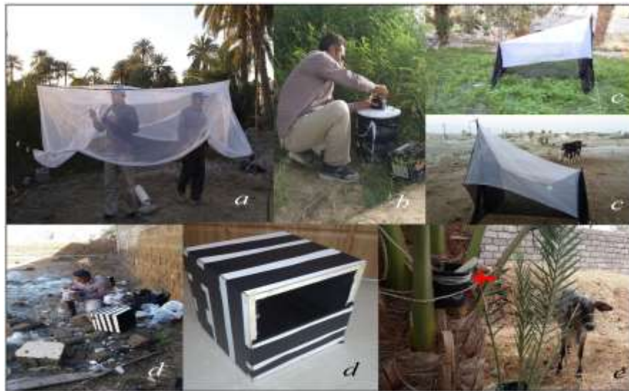
Fig. 2. Traps used for mosquito collection, CO 2 -baited bednet tarp (a), Malaise trap (b), 450 resting box (c), BG (d), ovitrap (e), southeastern Iran, Sistan and Baluchestan Province, 2016–2017
